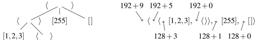
Figure 1: An example RLP tree and its encoding.
